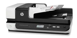
Scan resolution: Hardware: Up to  $600 \times 600$  dpi; Optical: Up to 600
