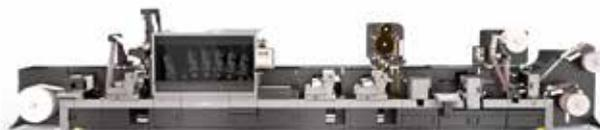
The LabelStream 4000 **HYBRID** configuration offers a custom mix of UV flexo, embellishment and finishing units, turning it into a fully integrated single-pass label conversion line. This mix of conventional and digital technologies enables a complete inline production of high-quality self-adhesive labels.
