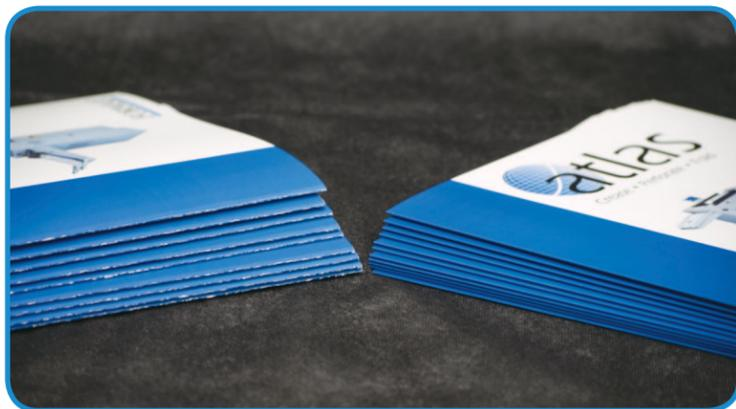
Uncreased folded digital prints (left) are cracked and give the appearance of poor quality. Creased prints (right) have no cracking and look polished and professional.
